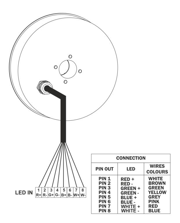
The maximum distance between DRIVENET PSU and DONUT 6 FC unit should not exceed 100 meters.
