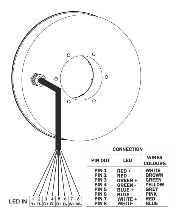
The maximum distance between DRIVENET PSU and DONUT 12 FC unit should not exceed 100 meters.
